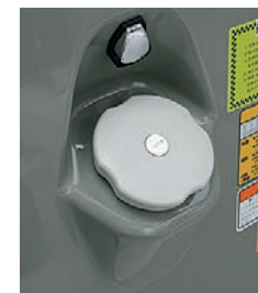
Fuel Port with lock
